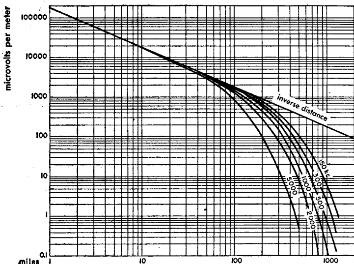
Fig. 3—Strength of surface waves as a function of distance with a vertical antenna for sea water ( \sigma = 4 \times 10^{-11} emu and \epsilon = 80 esu).
